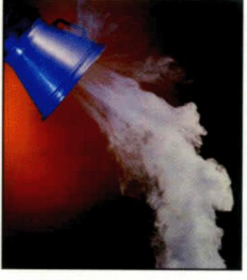
Standard hood design without parabolic shape and inlet flange allows smoke bypass.
